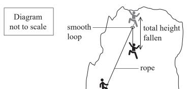
(a) The 'fall factor' is used by climbers to estimate the severity of a climbing fall and is given by
