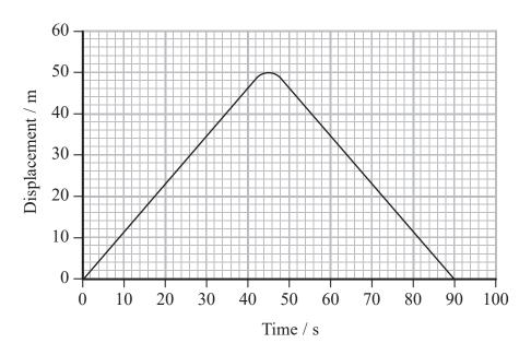
(a) Draw a corresponding velocity-time graph for the motion of the swimmer on the axes below. Show all working in the space below.
